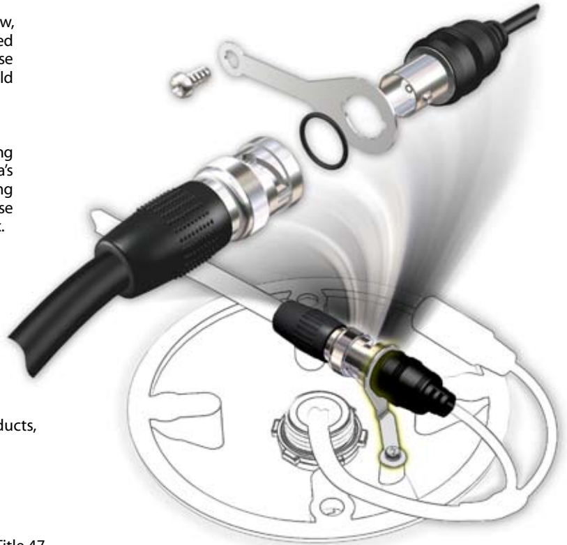
Figure 4 - Grounding the camera through the base with a grounded coax
