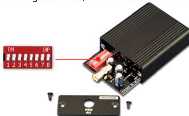
Figure 5 - UTP Decoder DIP Switches. Default of all OFF works for most installations. If necessary, start with #1 and turn more ON as the cable length increases; turn them all ON for the longest distance, 1000 feet.
